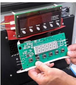
**6.** On the left side of the new board, attach the two wires supplied in the kit to the 2 connectors on the PC Board. Run the wires to the back of the heater on the same path as the original wires from the transformer.
