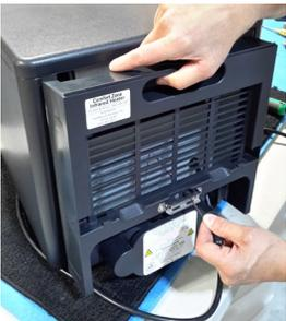
**9.** If you are sliding the heater back into a wood case, make sure that none of the wires on the new PC Board get pinched.
