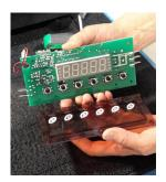
**5.** Now, remove the wires, one at a time from the right side of the old board and attach them to the new board in exactly the same order as they were on the old board.
