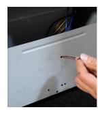
**8.** Next, reattach the plastic body panels and front cover. Guide the thermostat sensor through the hole in the plastic back panel and attach the sensor cover.
