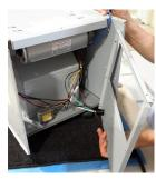
**2.** Disconnect the wires on the old board that go to the transformer.
